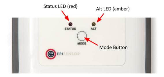
A node must be in "command mode" before users can interact with the product. To put the node in Command Mode, press and hold the "MODE" button for 2 seconds, then release. At this point, a battery powered node will switch the LED On Solid, while a mains powered node will flicker the LED and then switch the LED On Solid.
