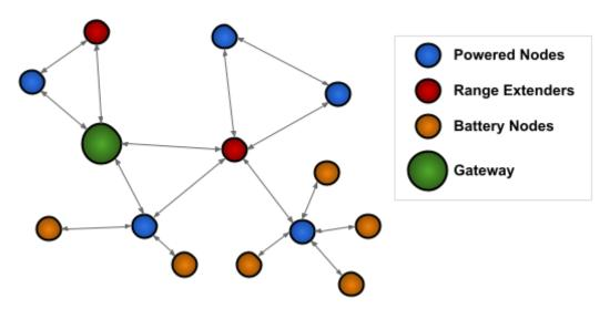
Range extenders are powered nodes where the main function is to route data. Any node with a mains power supply will act as a routing node in the network. Battery nodes do not route data – they spend most of the time in a low power mode.
