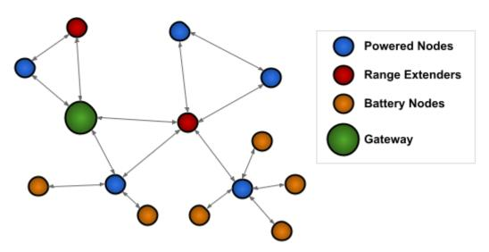
Range extenders are powered nodes where the main function is to route data. Any node with a mains power supply will act as a routing node in the network. Battery nodes do not route data – they spend most of the time in a low power mode.
