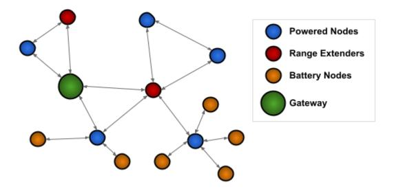
Range extenders are powered nodes where the main function is to route data. Any node with a mains power supply will act as a routing node in the network. Battery nodes do not route data – they spend most of the time in a low power mode.
