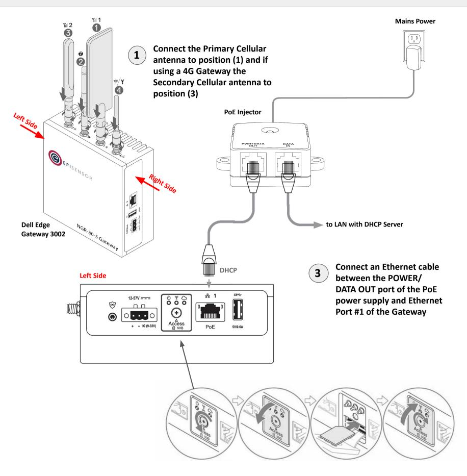
With the Gateway powered down, remove the screw from the access door and insert a micro-SIM as shown, then close the screw firmly.
