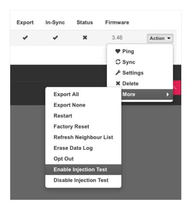
This will send a command to the ZDR, and the injection test will start on the next 15th minute.
