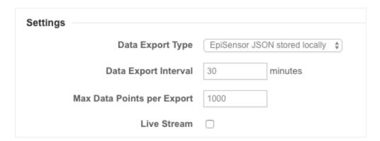
When the injection test has completed, data files that have been recorded will be available to download from the Data > Data File Archive page on the Gateway. Note that with the data export interval set to 30 mins, it could take up to 30 mins after the injection test has finished for all data files to be available for download.
