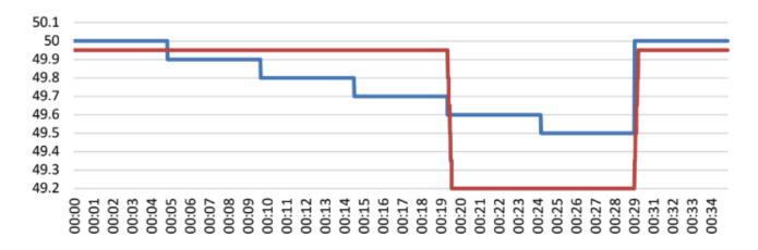
This profile will inject a line frequency as follows, and the test will last 35 minutes in total:
