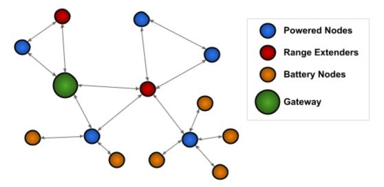
Range extenders are powered nodes where the main function is to route data. Any node with a mains power supply will act as a routing node in the network, and each node has a unique serial number which is used to uniquely identify it on the wireless network.
